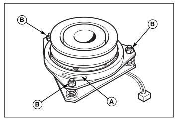
Figure 12. PTO Clutch Adjustment
